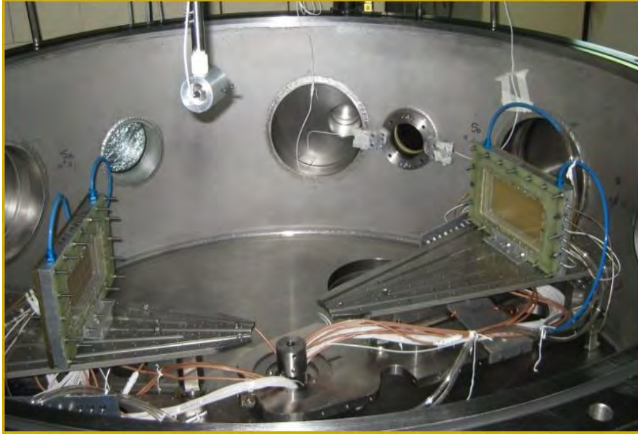
Fission fragment mass distribution measurement using MWPC time of flight set-up inside scattering chamber
