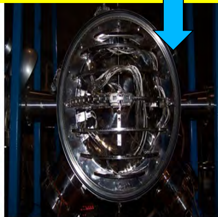
(b) Experiment using 10 nos of detector telescopes mounted inside the vacuum chamber.
